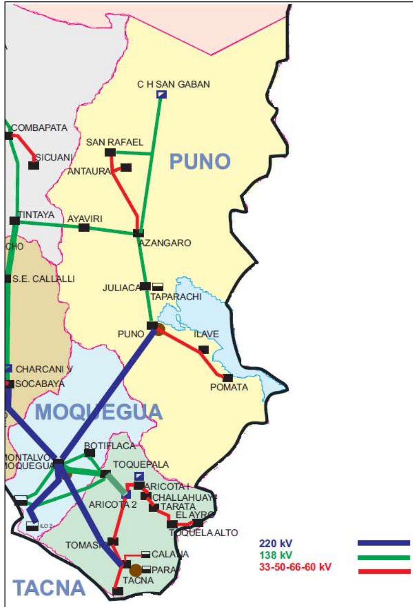
Figure 5-3: Southern Electric Ring Schematic
