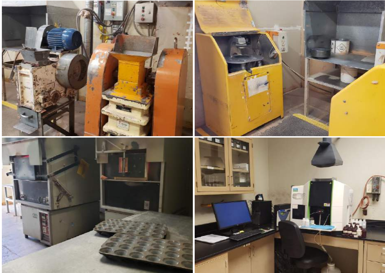
Figure 12-5: Mine laboratory: crusher (upper left), pulveriser (upper right), oven (down left), and ICP-AES (down right)
